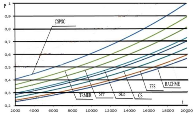
**Fig.1.** Probability of loss of operability of SPP subsystems
