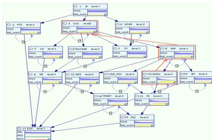
**Fig.2.** Scheme for searching for the cause of failure of the CSPSC subsystem in the diagnostic model of the technical condition of the SPP BBN
