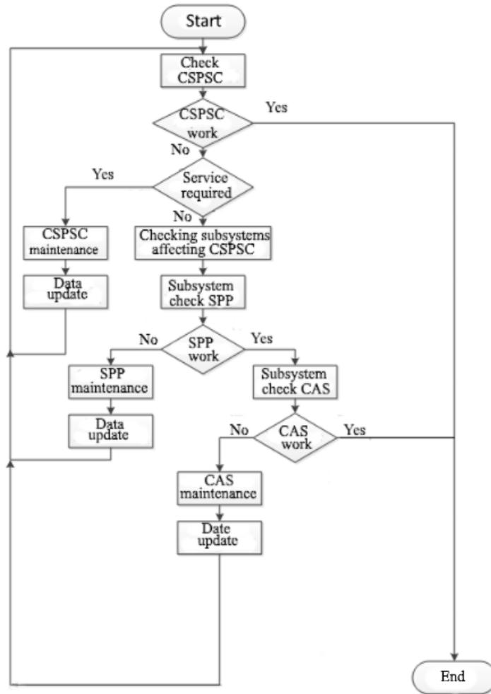
**Fig. 3.** Algorithm for troubleshooting the CSPSC subsystem
